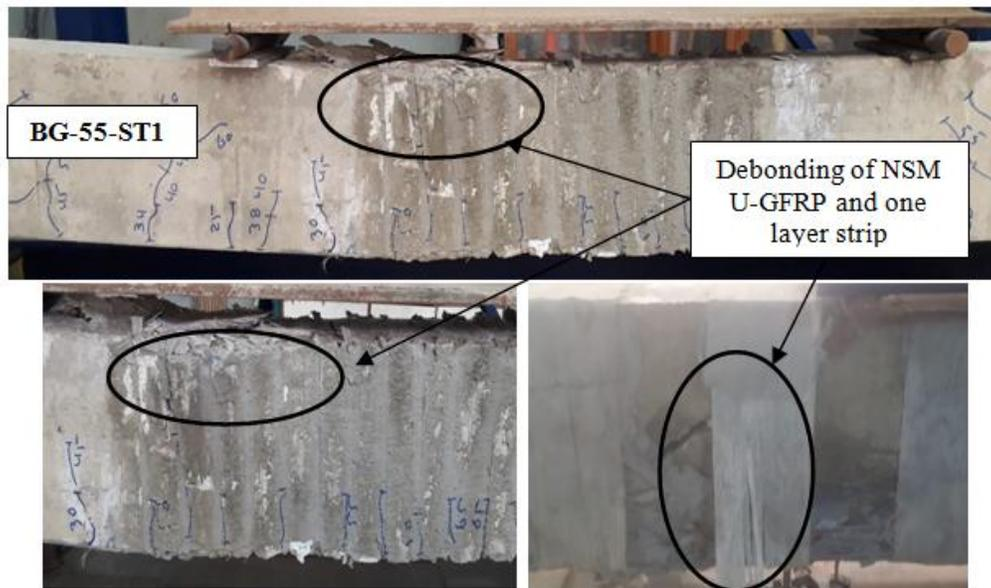
Fig. 6c. Typical de-bonding/flexural failure
