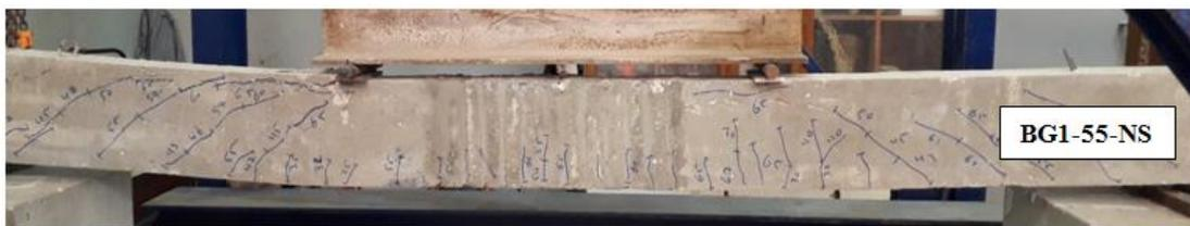
Fig. 6d. Typical ductile flexural failure for strengthened beams
