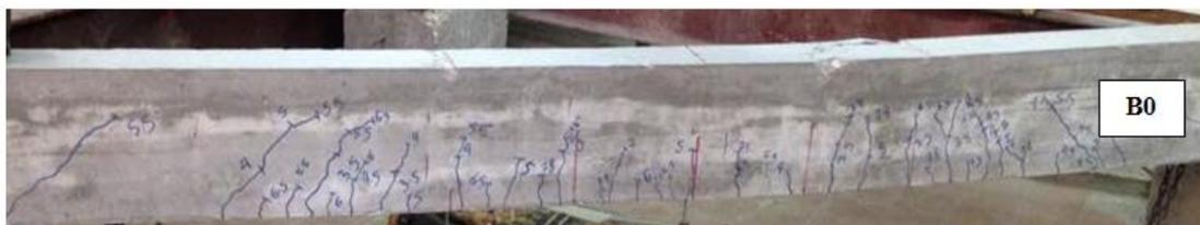
Fig. 6a. Flexural failure for B0 beam specimen without spliced
